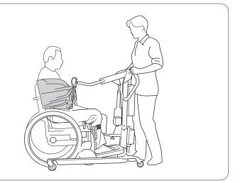
2. Connect the vest's straps to the sling bar's hooks. Tighten the calf strap.
