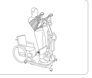
4. For a more upright position, continue the lifting motion to the uppermost position. The raising motion can be experienced as unpleasant for the person not used to it. Remember that Sabina II EE has two different speeds. For maximum comfort, the lift mast should be affixed to the base in the best possible of the three fastening holes. See page 5.
