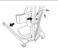
Manual base-width adjustment (Sabina EM) Base-width adjustment is done by pushing the lever backwards out of the blocked position and sideways to adjust the width. When the lever is released, the position is blocked.
