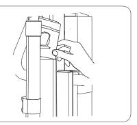
12. Place the quick reference guide in the holder on the lift mast.
