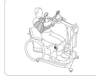
3. Raise the sling bar about 10–20 cm (4-8 in). The patient grabs the sling bar. Continue the lifting procedure. If the patient leans backwards, the raising will be made easier, preventing the vest from sliding up. The height to which the lift should proceed varies from person to person.
