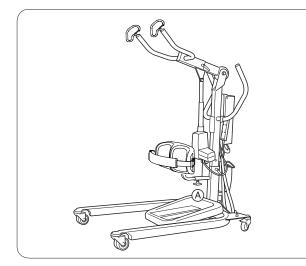
1. Disassemble the lower leg support: Unscrew screw A. Pull out the lower leg support. Remove the foot rest: Grab the front edge of the frame. Fold it up and lift it off the base.
