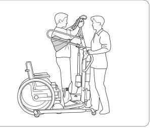
4. Continue the raising motion to the height desired. The SideSupport provides good support in the standing position.
