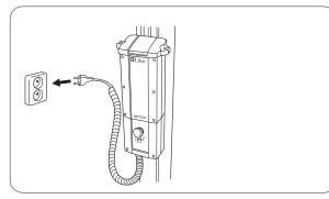
13. Before the first use, the lift's battery should be charged for at least 6 hours. For detailed instructions, see "Charging the Batteries", p. 8.
