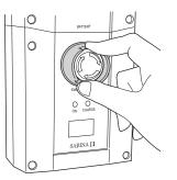
11. Release the emergency stop by turning the button in the direction indicated by the arrows on the button.
