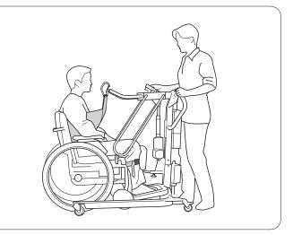
2. Place the SupportVest around the patient in accordance with the vest's instruction guide. Connect the vest's straps to the sling bar's hooks. Tighten the calf strap.
