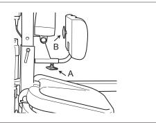
9. Install the lower leg support on the lift mast. Loosen wheel A in order to adjust the distance to the patient's
