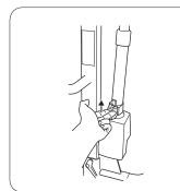
Mechanical emergency lowering Pull the red emergency lowering control straight upwards. Mechanical emergency lowering only works when the lift arm is under load, i.e. when a patient is standing/sitting in the lift. The lowering motion is slightly delayed.
